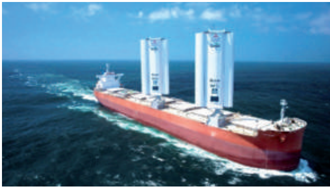
Figure 1 Pyxis Ocean bulk carrier fitted with two rigid wing sails to reduce fuel consumption (©CHEK project/Cargill)
