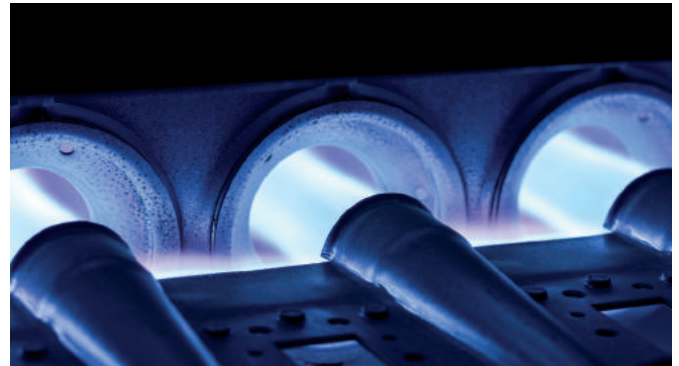
Example of horizontal, natural gas-fired burners in operation
