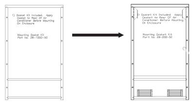
3) Apply gasket kit(28-1056-06) to adapter plate(28-2308-00). This gasket will be "sandwiched" between the adapter plate and the enclosure.
