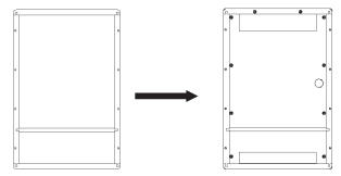
4) Apply adapter plate to unit using 10 screws.
