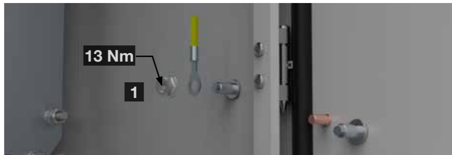
1 Flange nut serrated M8
