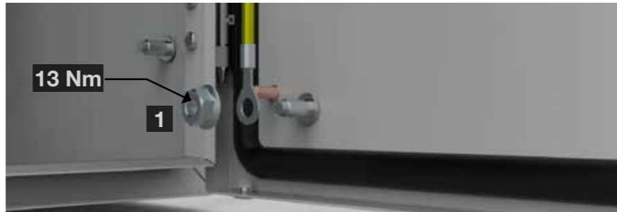
1 Flange nut serrated M8
