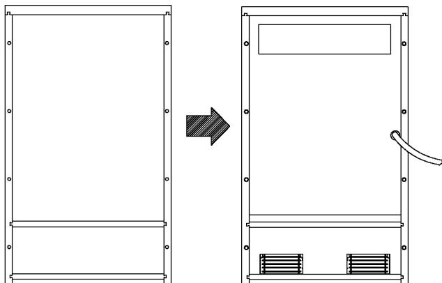
3) Apply gasket kit (28-1056-07) to adapter plate (28-2321-0X). This gasket will be "sandwiched" between the adapter plate and the enclosure.
