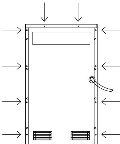
2) Apply gasket kit (28-1000-50) to rear of unit. Be sure the holes in the gasket align with the holes in unit. This gasket will be "sandwiched" between the unit and adapter plate.
