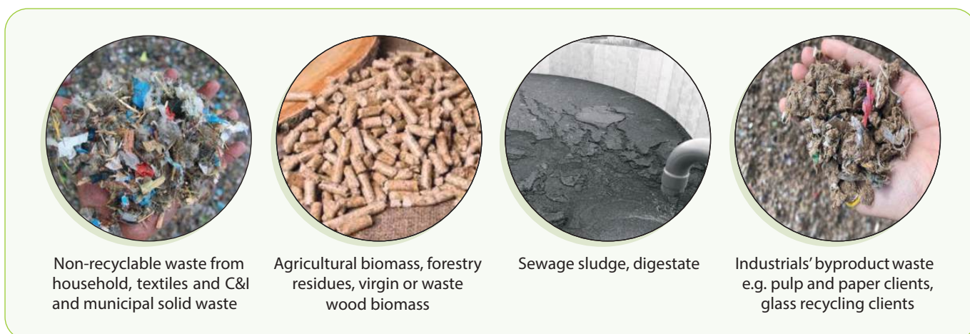
Figure 4 A variety of feedstocks can be used for gasification
