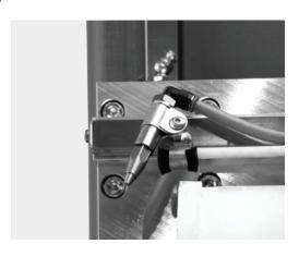
Minimal lubrication system extends tool life without creating a mess.
