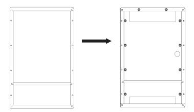
3) Apply adapter plate to unit using 8 bolts and 2 screws.
