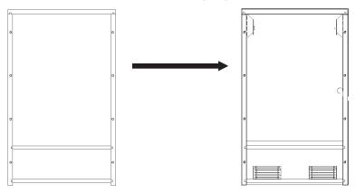
2) Apply gasket kit(28-1056-06) to adapter plate(28-2308-00). This gasket will be "sandwiched" between the adapter plate and the enclosure.
