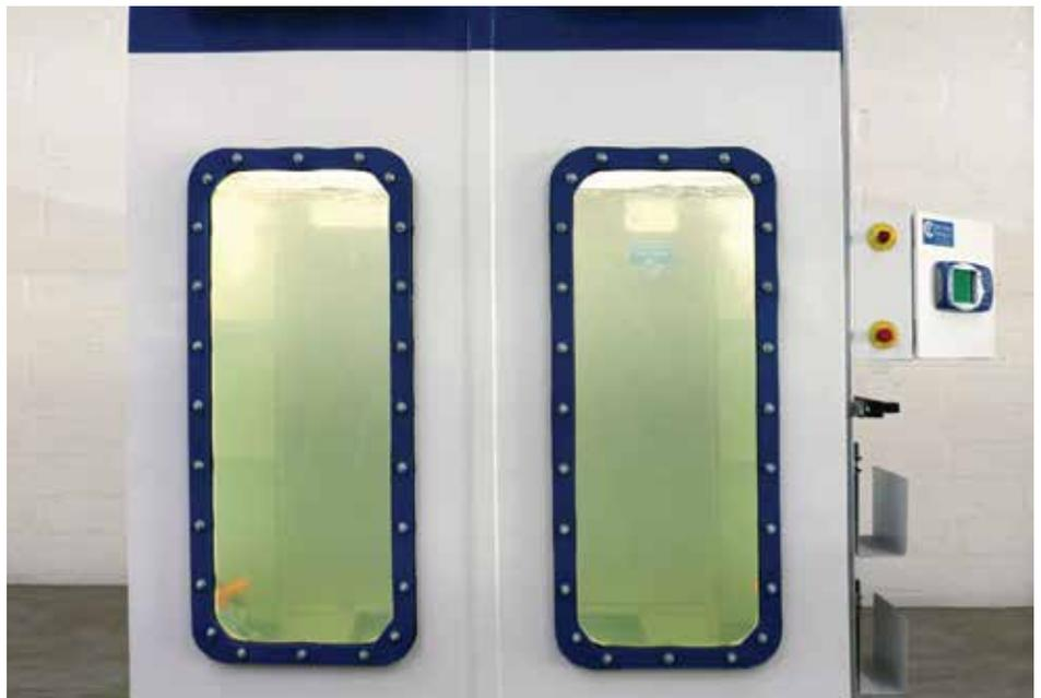
Testing for submersible application of nVent HOFFMAN Freestand enclosure at CCT
