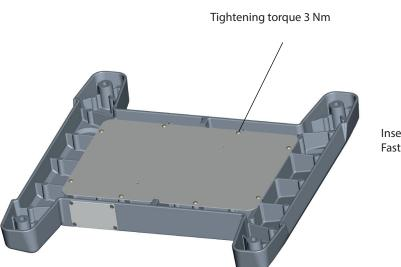
Insert the locking plate Fasten plate with 8x M5x10
