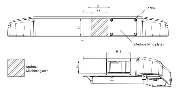
Maximum cover surface determined by opening behind interface blind plate
