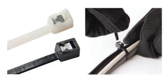
The nVent CADDY Self-Cutting Cable Tie is a versatile, tool-free datacom and general bundling solution for large amounts of cable. This simple, yet innovative product features a built-in cutting blade to ensure a secure fastening and a safe, clean tie-off finish. Made from durable 6/6 nylon, the Self-Cutting Cable Tie boasts a robust 22 kg of tensile strength.
