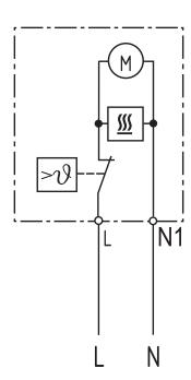
Heating units are used to prevent the development of condensation and drops in temperature in control cab-inets. Heating units must only be used in fixed, closed control cabinets. Heating units without an integrated thermostat should be connected in series to a suitable thermostat for temperature control.
