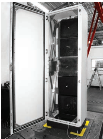
Figure 8. MCS20088R5 With seismic kit, seismic plinth and loaded mounting plate.
