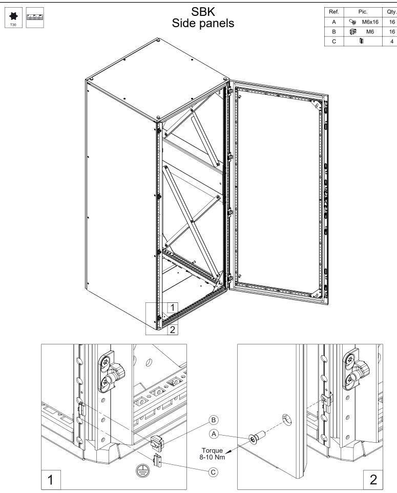
NOTE: Remove the retainers from side panel befor instalation
