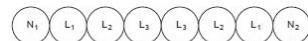
Figure H.52.1 – Special configuration for 6 parallel single-core cables in a flat plane (see 523.7)
