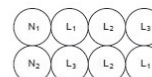
Figure H.52.2 – Special configuration for 6 parallel single-core cables above each other (see 523.7)
