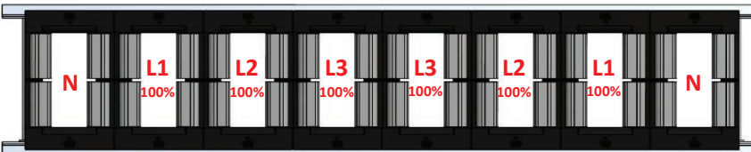
Optimized Conductor Arrangement (Load current balanced)
