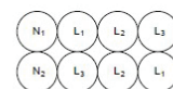
Figure H.52.2 – Special configuration for 6 parallel single-core cables above each other (see 523.7)
