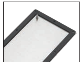
Full-size gland plate 3mm thick (12 gauge) flat bottom gland plate with bonding stud and continuous gasket seal
