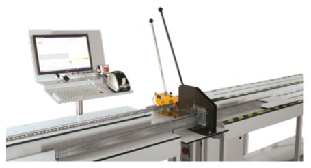
User simply feeds material until it reaches the motorized stop and then operates the shear manually.
