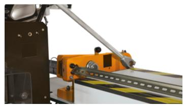
DIN rail and busbar cutting is accurate and easy.
