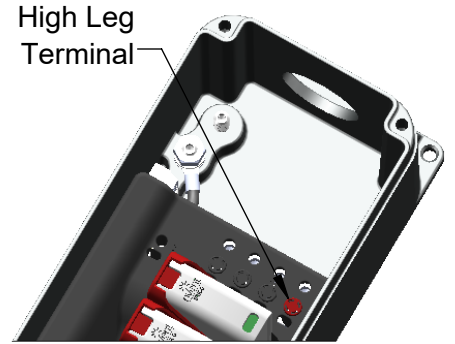
Figure 3: High Leg Identification
