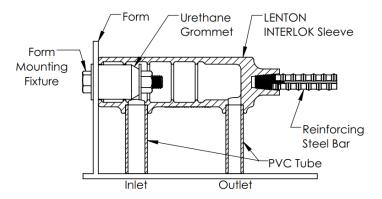
**NOTE!** It is recommended that grout tube lengths be kept to a minimum to ease job site installation of LENTON INTERLOK HY15LM grout. Slight bending of PVC tubing may be required to ensure proper installation of grout tubes. Temporarily plug access to grout tubes to prevent debris from obstruction placement of grout at job site.
