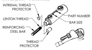
LENTON INTERLOK couplers are fastened to the rebar using a LENTON Tapered Threaded Bar End and placed into a pre-cast form. The LENTON INTERLOCK splice is completed at the jobsite by inserting the exposed dowels of an adjoining pre-cast member into the coupler grout cavities and filling with LENTON INTERLOK HY15LM Grout.
