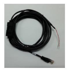
Enlogic's Dry Contact Cable is designed to monitor conditions such moisture detection, motion, door sensor, and access through external dry contact sensors. This allows for convenient control of vital datacenter and IT equipment with minimal effort quickly and efficiently. The dry contact cable can be extended (up to 30.5 m) using a standard RJ-45 coupling.
