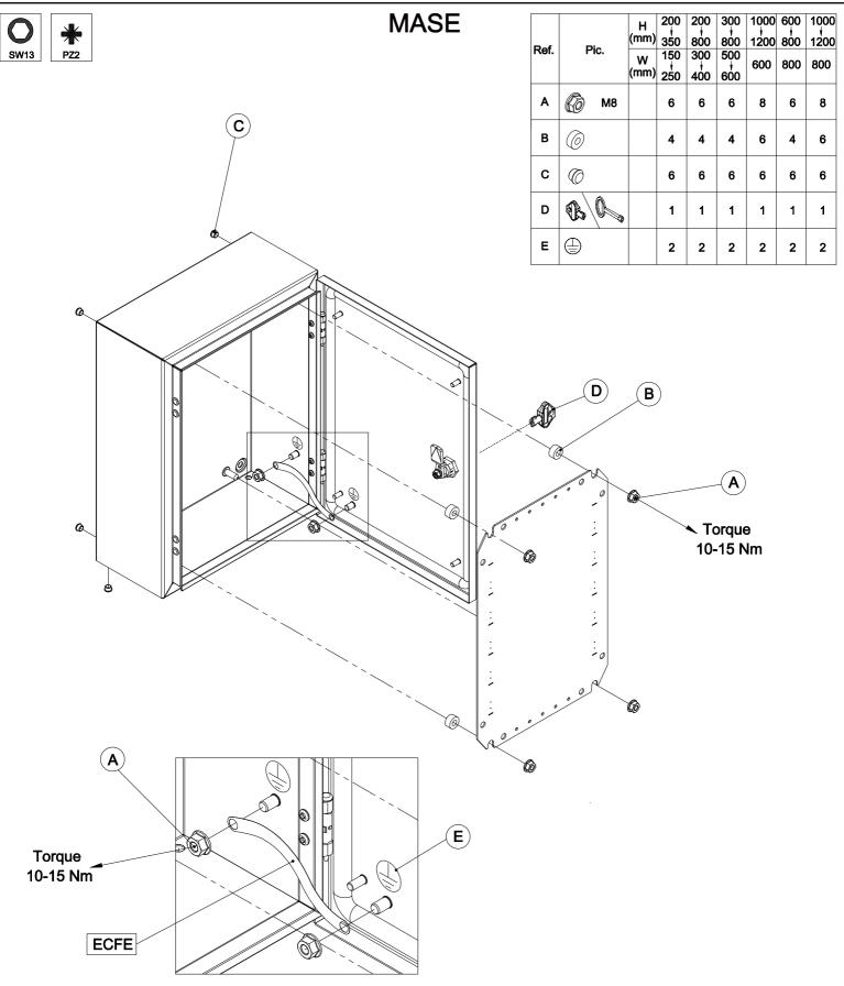
**WARNING:** When mounting on or over a combustible surface, a floor plate of at least 1.43 mm galvanized or 1.6 mm uncoated steel extended at least 150 mm beyond the equipment on all sides must be installed.
