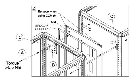
\* - Internal Baying brackets must be mounted before MM
