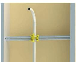
The nVent CADDY In-Wall Conduit Positioning Clip is an intuitive, tool-free and screwless solution to quickly and securely position 20 to 25 mm conduits onto nVent CADDY Telescopic Screw Gun Box Straps. Ideal for drywall installations taking place before electricians arrive onsite to wire electrical boxes — commonly known as "hockey stick" installations.
