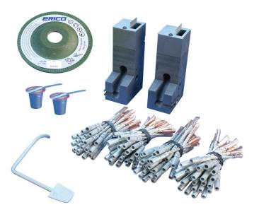
The nVent ERICO Cadweld Plus Rail Track Connector Bond Kit, Multi-leg, is intended to be welded to the web of the rail at the neutral axis. The kit has all the necessary components to establish a welded bond connection to the web of the rail. To ensure connection integrity, the attachment shall be made using nVent ERICO Cadweld Plus welding material. The multileg track connector was developed to allow multiple connections in tight spaces while maintaining rail integrity.
