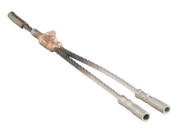
The Rail Track Connector Bond, Multi-Leg is designed for rail wayside signaling applications. This solution is designed to allow multiple connections to rail in highly congested areas of track while safely maintaining rail integrity. Connections to the rail can be made via nVent ERICO Cadweld exothermic connection or nVent ERICO plug bond connection.
