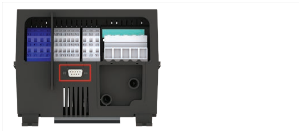
Figure 11 - Profibus Interface on Elexant 4020i Variant
