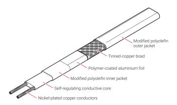
The nVent RAYCHEM HWAT self-regulating heating cables maintain the desired water temperature in a building's hot water distribution pipe network.
