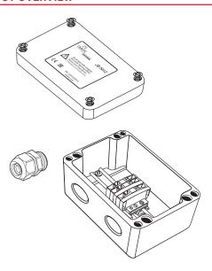
The nVent RAYCHEM JB-NH2 is a non-hazardous junction box for use with various heating cable types with M25 connection kits.
