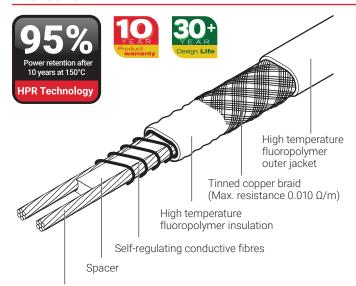
2.3 mm<sup>2</sup> nickel plated copper conductors
