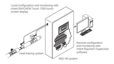
The nVent RAYCHEM NGC-40 is a multipoint electronic control, monitoring and power distribution system with a unique single-point controller architecture for heat-tracing used in process temperature maintenance and freeze protection applications. By taking advantage of innovative modular packaging techniques, the nVent RAYCHEM NGC-40 system provides configuration and component flexibility so that it may be optimized for a customer's specific needs.
