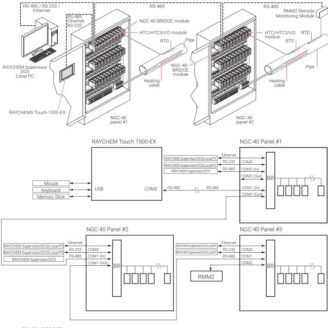
BR:NGC-40-BRIDGE DCS:Distributed Control System RMM2:Remote Monitoring Module
