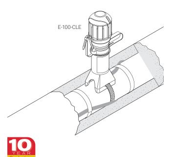
The nVent RAYCHEM E-100-CLE is an above insulation lighted end seal kit for nVent RAYCHEM 3, 5 and 8 XL-TRACE Edge cables in ordinary locations.
