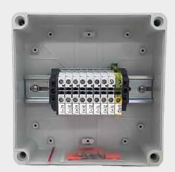
The Solar RU-2-LP Box enables installers to transition and/or combine one to four DC strings to a single conduit, reducing costs by enabling installers to switch to standard building wire and simplifying connections in the enclosure. The low profile enclosure is designed to be mounted beneath the array using the optional box bracket accessory or adjacent to the array using racking system accessories.
