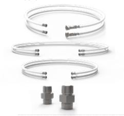
Flexible hoses to connect the cooler with facility coolant. Facility connection female BSPP 1" flat gasket. Cooler connection female BSPP 1" flat gasket or Danfoss FD83 quick disconnect couplers.
