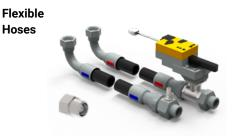
Flexible hoses to connect the cooler with facility coolant. Facility connection female BSPP 1" flat gasket. Cooler connection female BSPP 1" flat gasket or Danfoss FD83 quick disconnect couplers.
