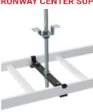
Threaded rod and bracket supports center of ladder rack from ceiling. Kit includes heavy-duty ladder rack cross member, two mounting brackets, two #12-24 screws, 5/8-in. threaded rod, protected sleeve and four 5/8-in. nuts. Use one kit at least every 5 ft. (1.5 m). Made of plated steel.
