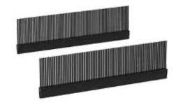
The ProLine S1 Brush Strip Kit provides a level of air flow management while providing a cable pass through. It has a single row of Nylon bristles attached to a flexible, black PVC mounting clip.
