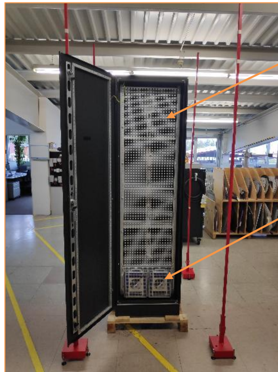
Figure 4 Noise measurement setup for LHX+ 10kW with open front door_Front View
