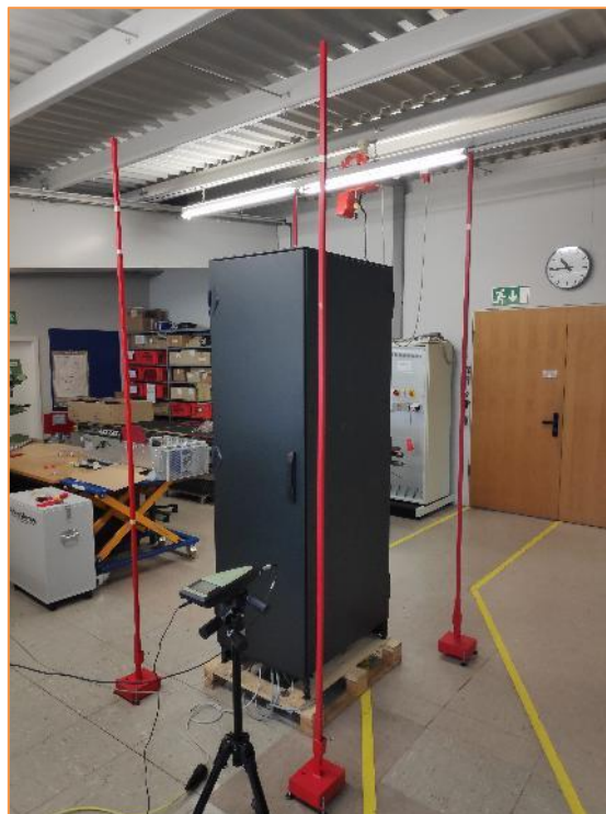
Figure 3 Noise measurement setup for LHX+ 10kW with closed doors_Rear view
