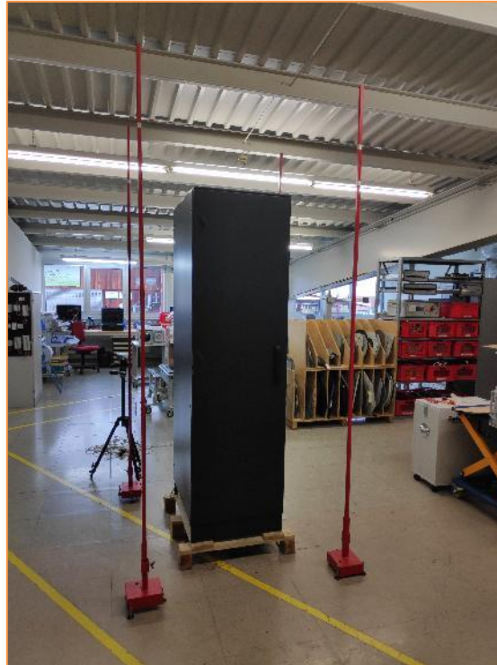
Figure 2 Noise measurement setup for LHX+ 10kW with closed doors_Front View
