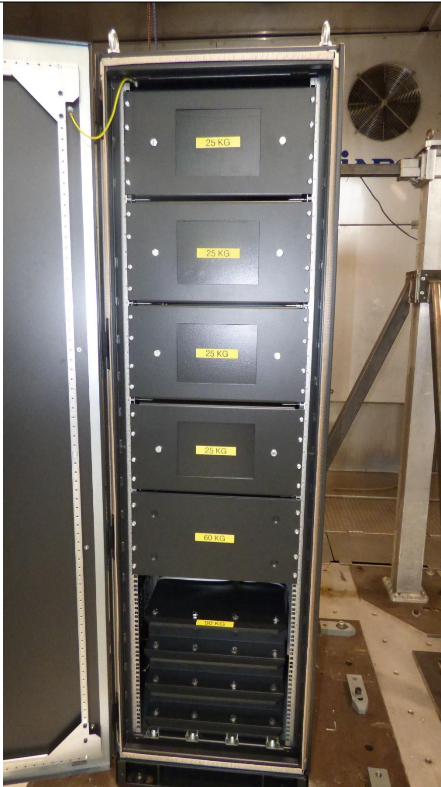
Figure 4: The cabinet with dummy weights (see Annex for weight distribution)
