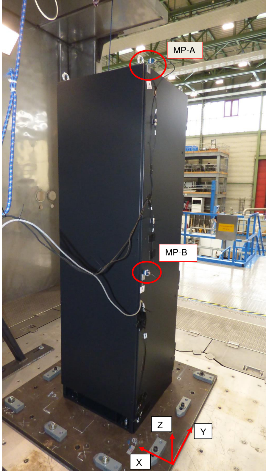
Figure 1: Test Setup and Measurement Points A-B; EuT rear view
