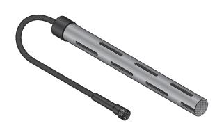
The nVent RAYCHEM TraceTek Fast Fuel Sensor (FFS) is designed to quickly detect hydrocarbon fuels floating on water or collecting in a sump. The probe ignores the presence of water, but reacts to a thin film of fuel floating on the surface. In most cases, the TT-FFS will reset when removed from contact with the spill and the fuel is allowed to evaporate.
