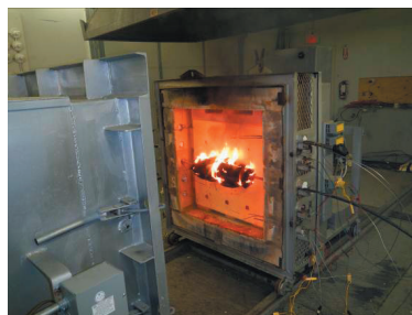
Enclosed furnace test for cable splice
