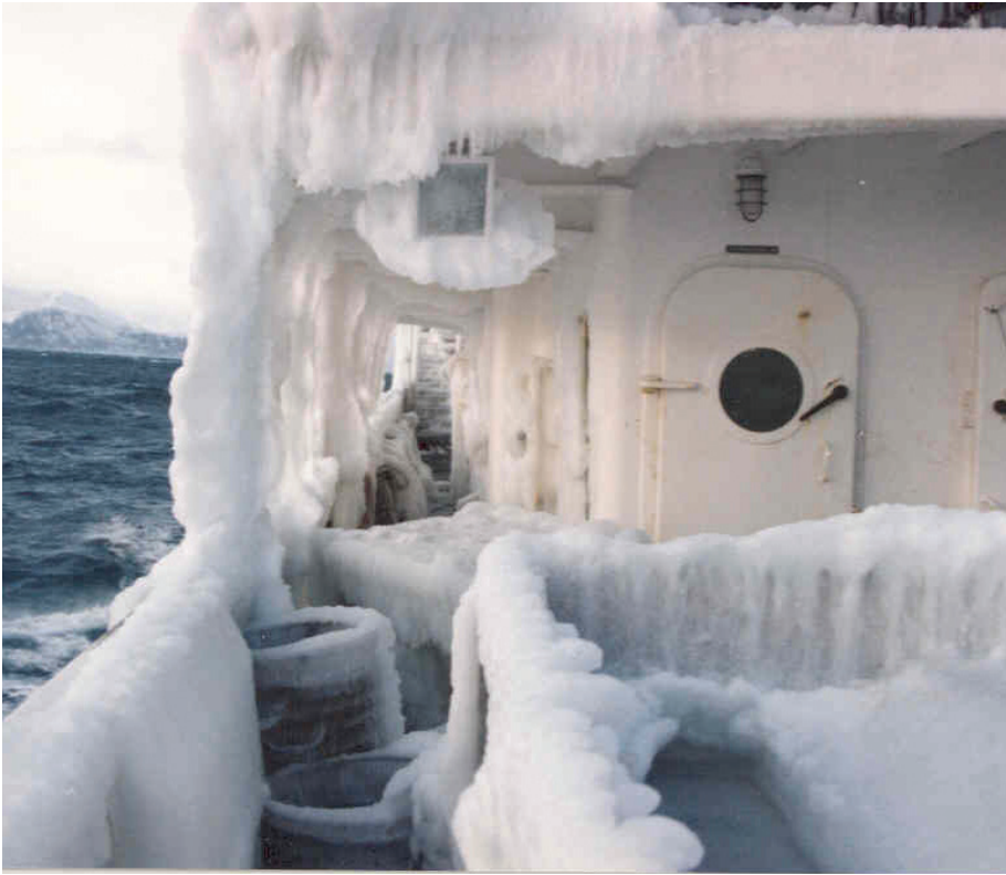
Figure 4. Example ice buildup on Essential Equipment.
