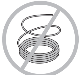
Figure 5: Unreeeling / uncoiling cable
