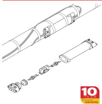
The nVent RAYCHEM S-150 is a cold-applied, low-profile splice for in-line connection. It is designed for use with the following nVent RAYCHEM brand heating cables: BTV, QTVR, and XTV. Use the S-150 in applications with temperatures ranging from  $-60^{\circ}$ F to 420°F ( $-50^{\circ}$ C to 215°C). It is approved by FM,CSA and Dekra for use in hazardous locations.
