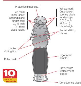
The nVent RAYCHEM Stripping-Tool-SR-Cable is designed for use with nVent RAYCHEM BTV-CR, BTV-CT, QTVR-CT, XTV-CT, HTV-CT, HWAT, XL-Trace, IceStop and RaySol self-regulating heat-tracing cables. The tool is designed for faster, safer and more reliable cable terminations.
