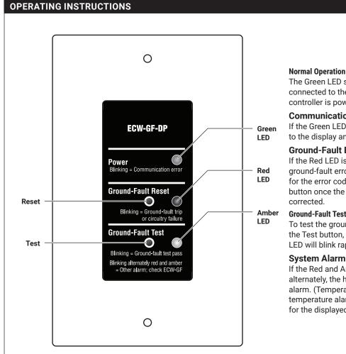
The Green LED shows that the display is connected to the ECW-GF controller and the controller is powered.
