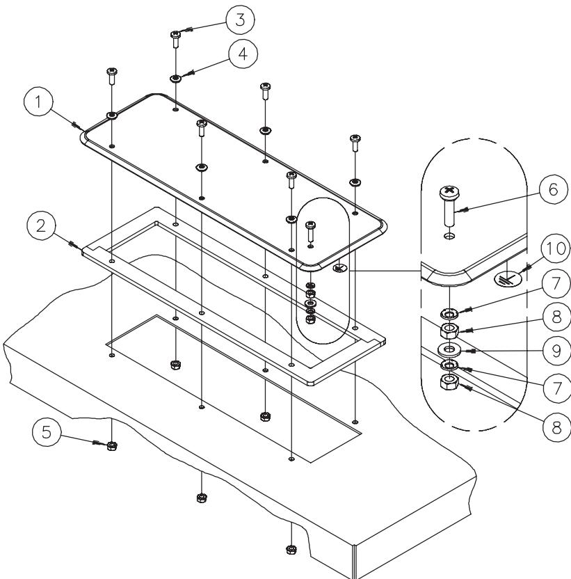
Maintains Type 4 and 12 when mounted on outside of enclosure.
