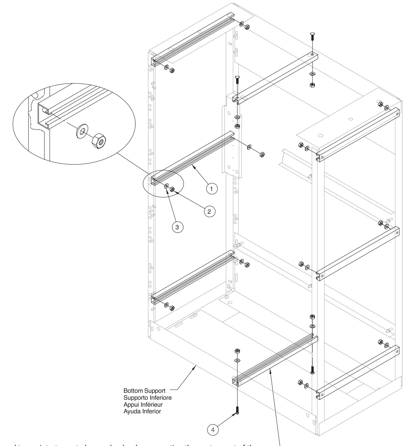
Bottom and top unistruts are to be used only when mounting the center post of the swing panel assembly. When using the bottom and top unistruts, the bottom support (A17SUPPORT2) must be installed (order separately).
