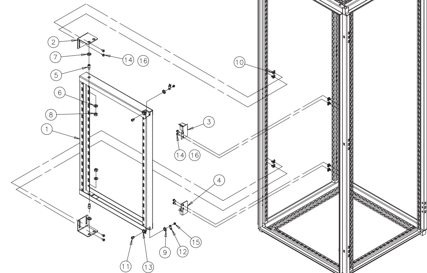
NOTE: The swing frame can be mounted using the M5x10 self-tapping screws (item 14), or it can be mounted using the M6x16 screws (item 16) with the M6 cage nuts (item 10).
