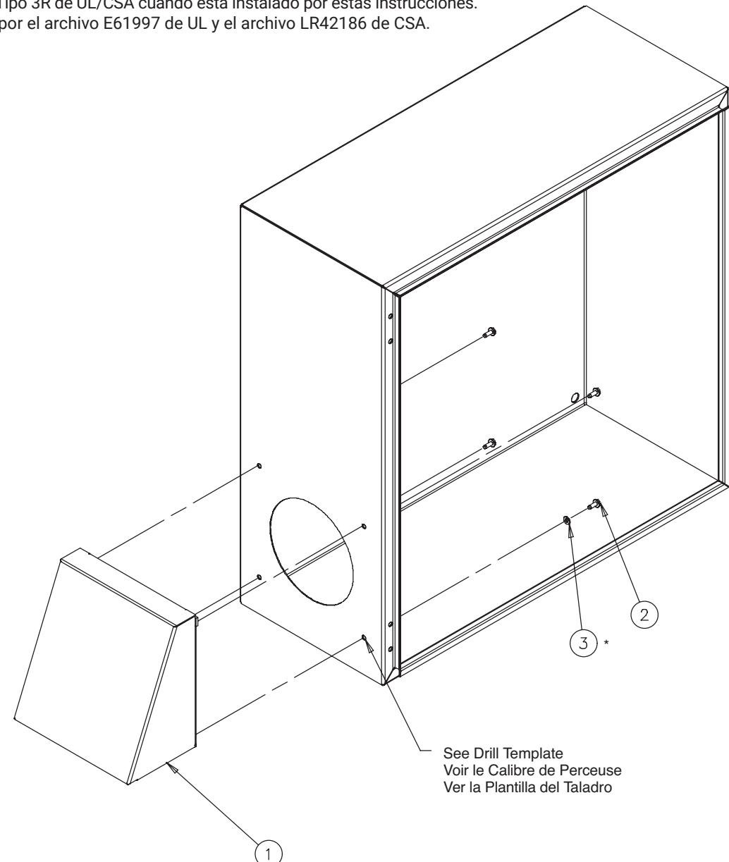
NOTE: 1. To avoid any component interference, lay out the drilling locations for the shroud before cutting any holes. The enclosure opening inside the rain shroud should be as high as possible and centered left-to-right.
